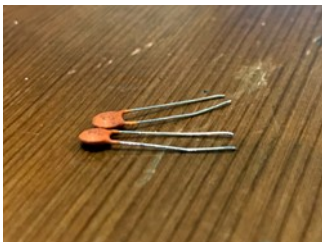
22pF Ceramic Capacitors Markings: 22
